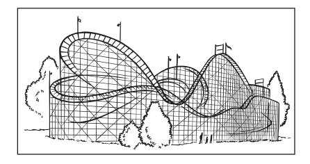
The rollercoaster at Play Land in Vancouver was built in 1958 and is the one of the oldest wooden roller coasters still in use in the world. Most roller coasters are made of steel. Another interesting fact about this rollercoaster is that after the initial ascent, the entire rollercoaster is completely powered by gravity only, which is intense. If you have ever ridden on it, you will know how fast it rips up and down those tracks. It speeds along at up to 75 km/h.
