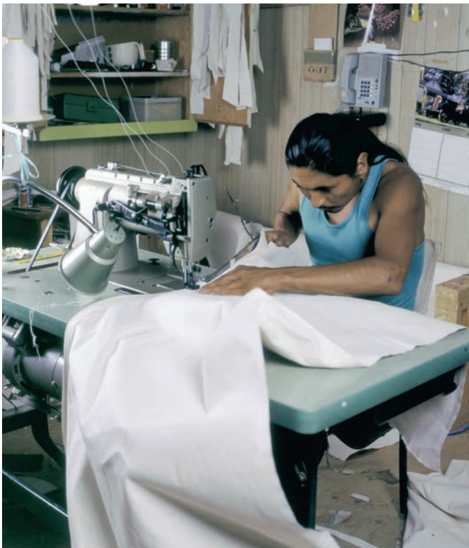
Richard Jacobs making a tipi for the Ktunaxa Tipi Company near Creston. Traditionally most Ktunaxa (Kootenay) people used animal hides for tipi covers, but in the Lower Kootenay area, reeds or rushes were sewn together. Today canvas is used and the tipis are double-stitched and have interlocking seams. A finished tipi is shown on the right.
